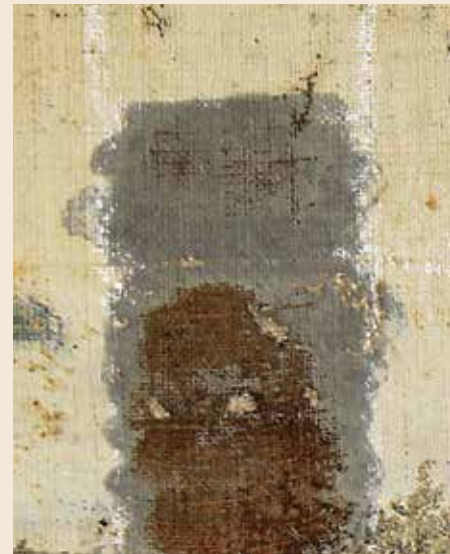
Fig. 4: Stages of laser treatment, from top: lead white before ablation, gray intermediate, complete removal.
