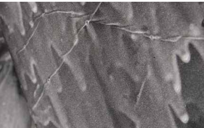
Detail of stearic acid "bloom" caused by crystallized fats in the oil-based paint.
