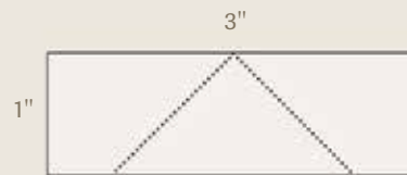
Step 1: Start with a strip of archival paper. Height of strip will determine corner size.
