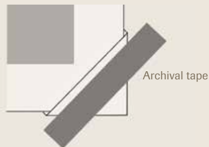
Step 4: Tape corner in place. Tape should not come into contact with print.
