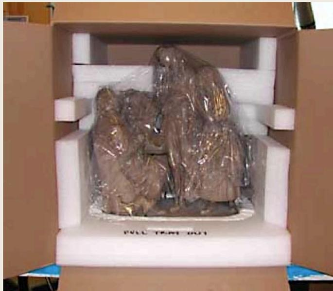
PE foam cutouts and bottom pull-out tray lined with cross-linked PE foam sheet; clear polyester sheeting wrap and double-wall corrugated box
